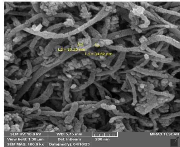
FE-SEM for MWCNTs-Tetra@Fe 3 O 4
