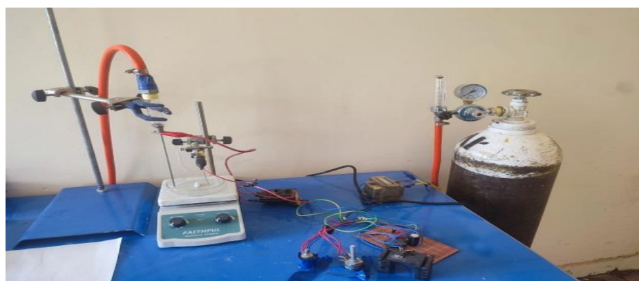
Figure 1 The diagram of atmospheric plasma jet electrochemical production of ZrO 2 nanopowder
